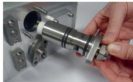
Totally serviceable from the header front
