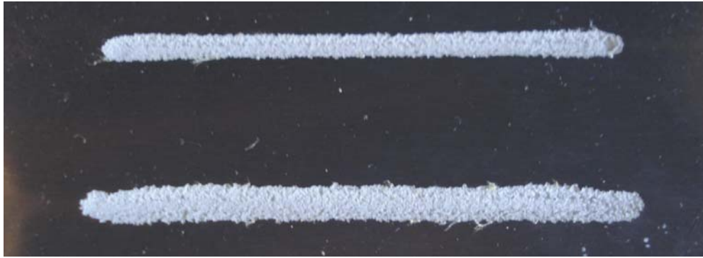
Fig. 16: Spray impact erosion comparison, Scalemaster Superior top, Scalemaster bottom
