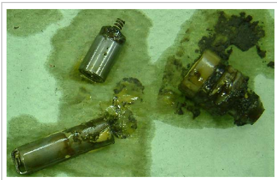
Fig 13, contaminated valve components
