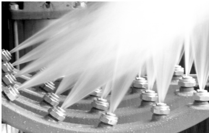
Figure 4 – Spray header with flat jet nozzles for roll cooling in section mills.
