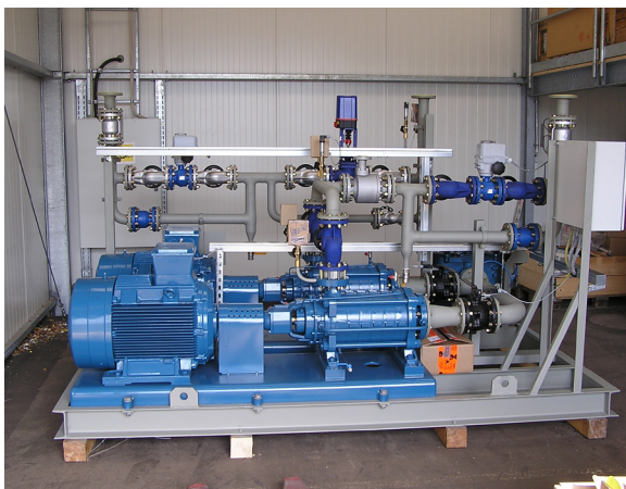
Pump and control skid preassembled.
