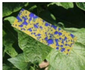
Wetting in the middle plant area
