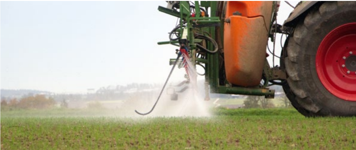
Optimum wetting thanks to twin flat spray jet
