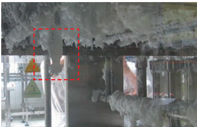
Figure 7: Foam cleaning with a Lechler PVDF MicroWhirly
