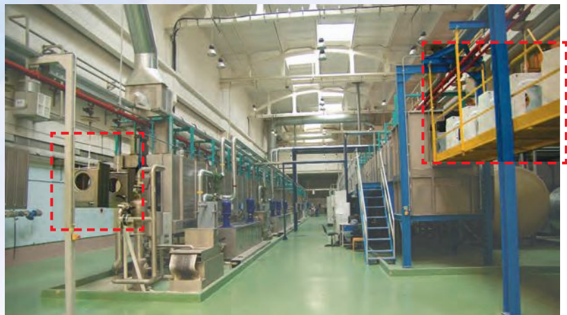
Example of a painting line for washing machine housings. On the left the component before painting, on the right the painting housing exits.
