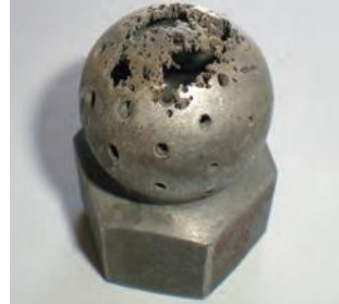
Fig. 1: Chemical corrosion of a spray ball
