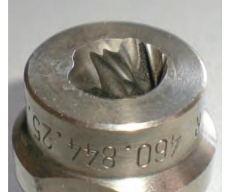
Fig. 2: Wear of a full cone nozzle ball
