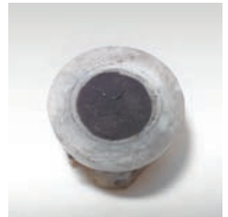
Clogged nozzle (back side)
