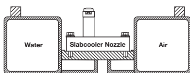
Example of Lechler air mist header design without cover plate on
