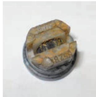
Clogged nozzle (front side)
