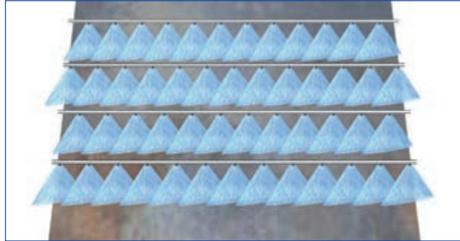
Example of a staggered nozzle arrangement
