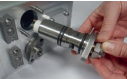
Totally serviceable from the header front
