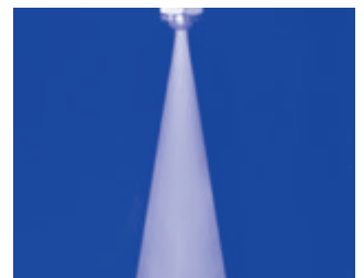
Spray pattern of the Laval nozzle
