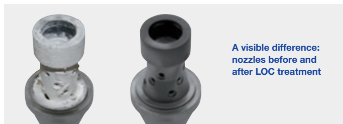
Cyclical cleaning with citric acid doped in compressed air
