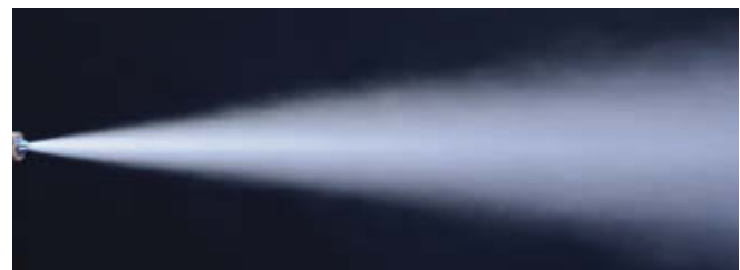
Spray pattern of a Laval nozzle
