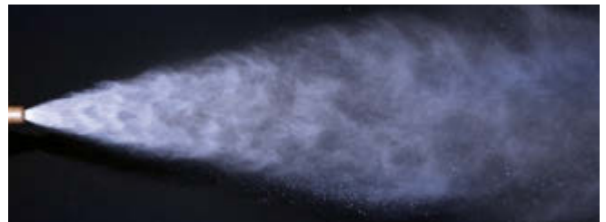
Spray pattern of a MasterNOx ® nozzle 30°
