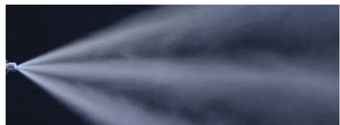
Spray pattern of a flat fan nozzle
