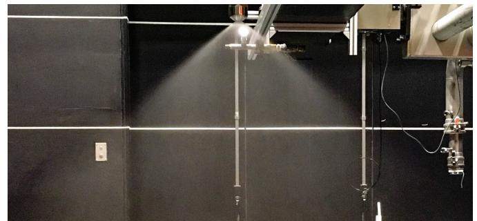
Spillback line open (min. injection), spray angle approx. 100°
