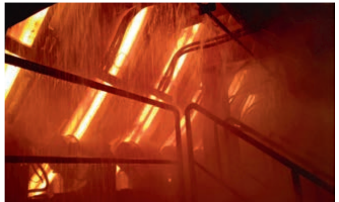
Secondary cooling zone of billet caster
