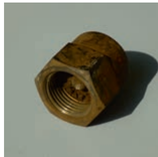
Clogged vane of a full cone nozzle
