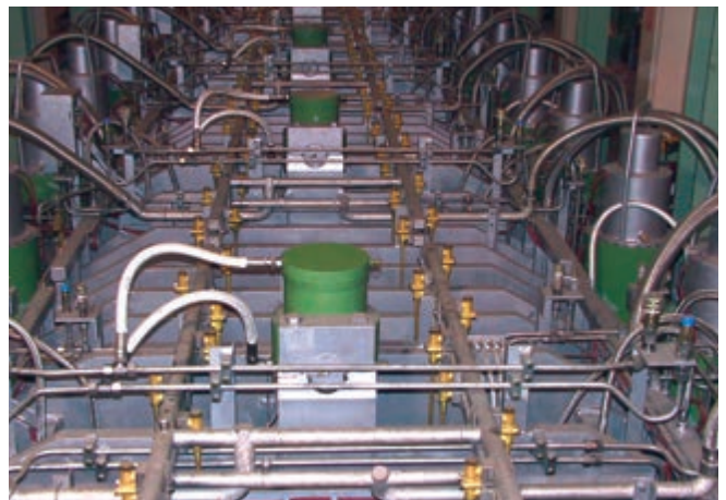
Horizontal segments with Mastercooler SMART nozzles
