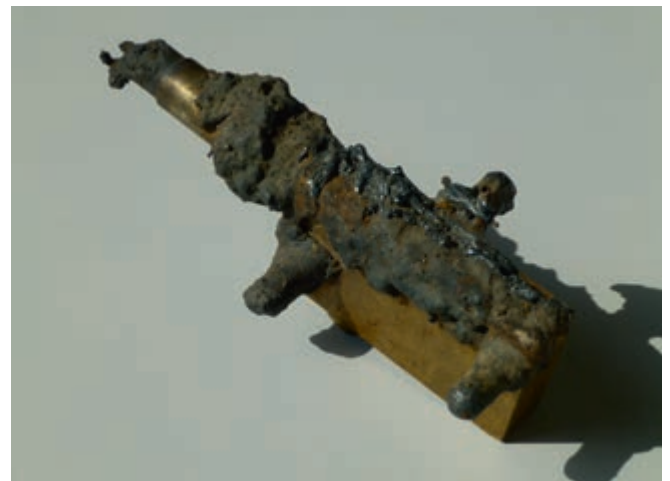
Air mist nozzle after break out of liquid steel
