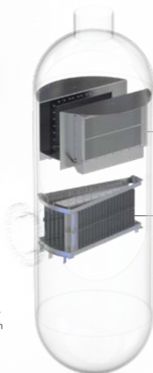
Arrangement of four droplet separators in a pressure tank
