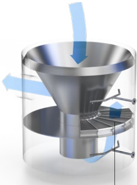
"Cake Piece" separator in an evaporator
